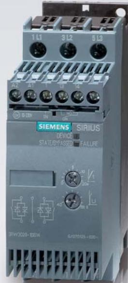
They protect the machine's mechanical power-transmitting elements during start-up through reduction of the starting torque and efficiently guard the network against excessive inrush peaks through reduced power input: the electronic soft starters 3RW30. Switchover current or torque peaks typical of star-delta starters are reliably excluded.
