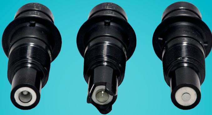
Process electrodes designed for general use built with durable, robust bodies with process connections (NPT threads or ISO threads) built in. These sensors are suited for continuous monitoring and controlling of pH or ORP in a wide range of light/moderate duty applications.
