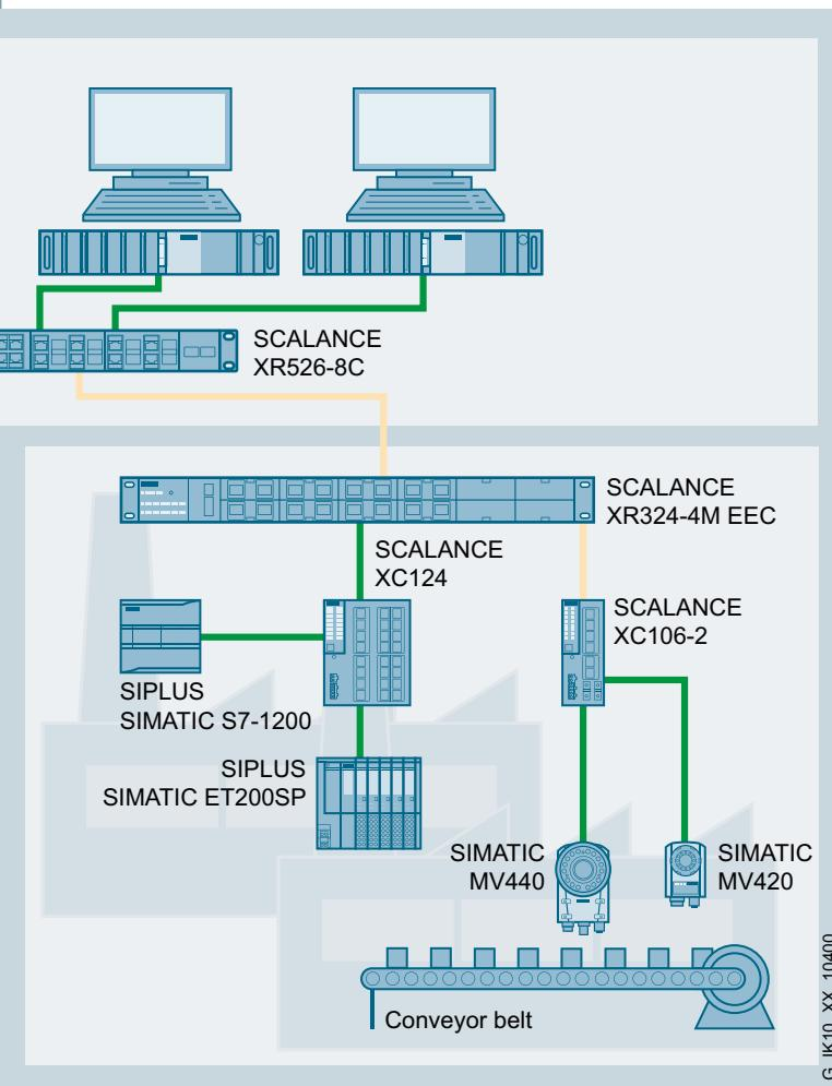
SCALANCE XC-100 in all its versions with different numbers of ports enables small networks to be constructed with the right switch for the respective application, e.g. for hazardous zones (IECEx, ATEX Zone 2). The available density of ports helps to save costs. In addition, all SCALANCE XC-100 devices undergo a Highly Accelerated Life Test (HALT). This involves subjecting the products to extreme overload test cycles to determine weaknesses in materials and design in an "accelerated lifecycle".
