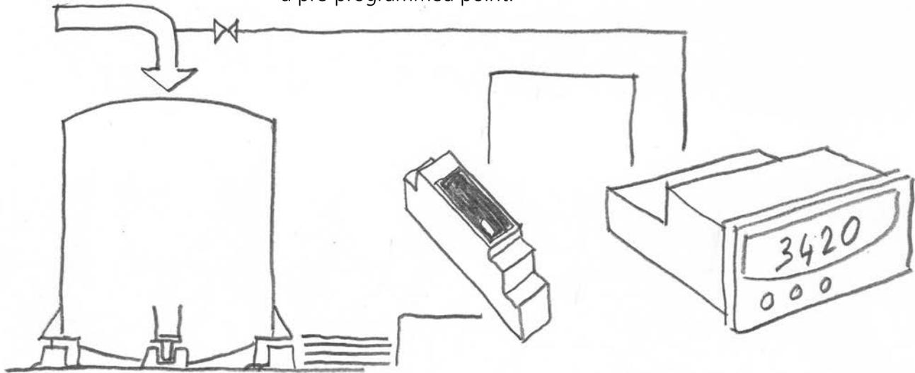
FOUR LOAD CELL INPUTS
