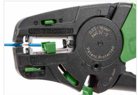
Partially stripping a conductor.
