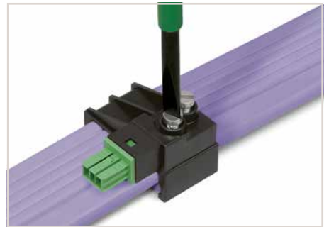
Tighten the screws to connect the flat cable. Observe 1 Nm of tightening torque!
