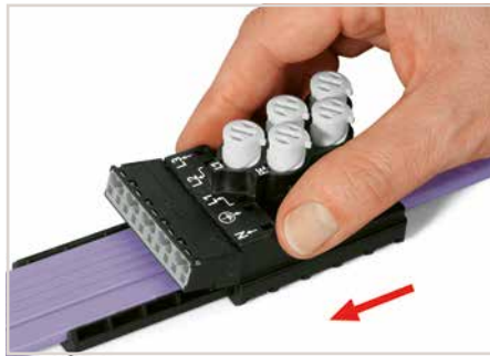
Mount IDC module flush with the base. Should the IDC module jam during mounting, turn the upper part by 180° and remount it.
