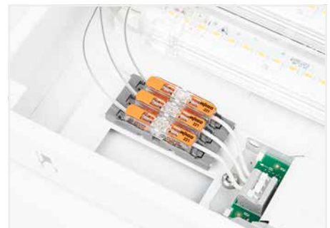
Multi-pole, fixed lighting fixture wiring
