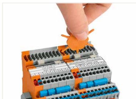
Insert coding pin into the corresponding slot and twist it off.
