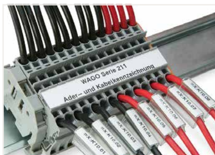
Slide the marker into the marking sleeve receptacle. Replacing the marker is also possible after the conductor has been terminated.
