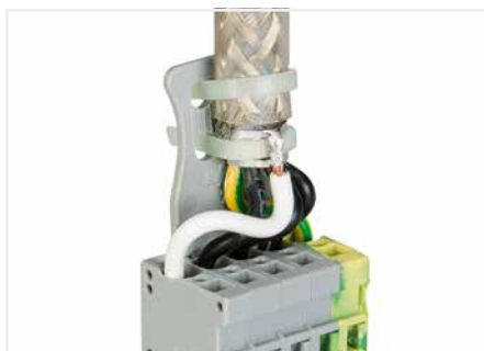
Secure both shield conductor and shield termination (790-350) to the strain relief plate using cable ties.
