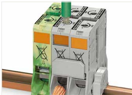
Conductor termination (50, 95 and 185 mm 2 ) – step 2 Insert a stripped conductor into the clamping unit until it hits the backstop. Hold in this position.
