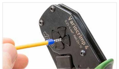
Inserting a ferruled conductor into the crimping station.
