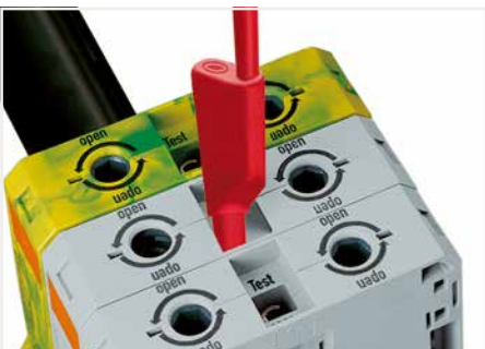
Easy troubleshooting via 4 mm Ø touch-proof test plug. A test plug adapter (283-404) is used for the 35 mm 2 (2 AWG) terminal block. (Test plugs are not available from WAGO, but are offered by industry suppliers such as Multi-Contact Deutschland GmbH.)
