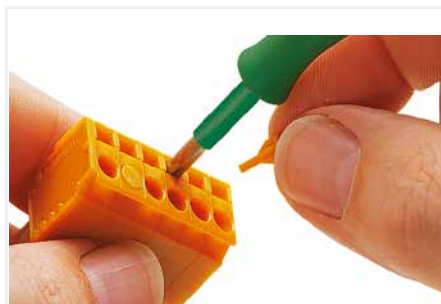
Covering unused clamping units in CAGE CLAMP®-equipped male and female connectors (e.g., when doubling the pin spacing to meet clearance and creepage distance requirements, or when a higher rated voltage is required). Lockout pins are not suitable for panel-mount, angled female connectors.
