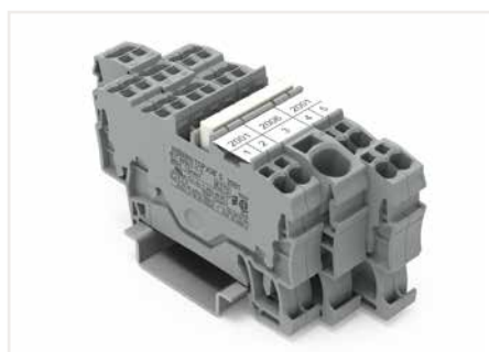
Increasing the number of output terminals of the distribution terminal block via commoning to suitable through terminal blocks.
