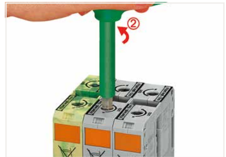
Conductor termination (50, 95 and 185 mm 2 ) – step 3 A short counter-clockwise rotation ② releases the tab. When unlocked, the T-wrench rotates clockwise, securely clamping the conductor.
