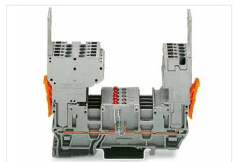
2-conductor and 1-conductor female plugs (may be reversed) LED carrier terminal blocks can be commoned via 280 and 780 Series Jumpers and tested using a test plug adapter (280-4..).
