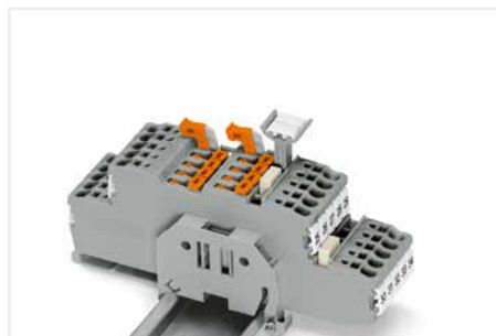
Double-deck, double-disconnect terminal blocks (2002-2951) with group marker carrier accommodated in jumper contact slot
