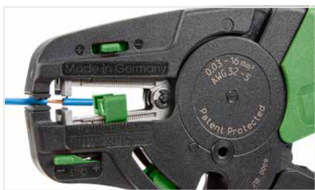
Partially stripping a conductor.
