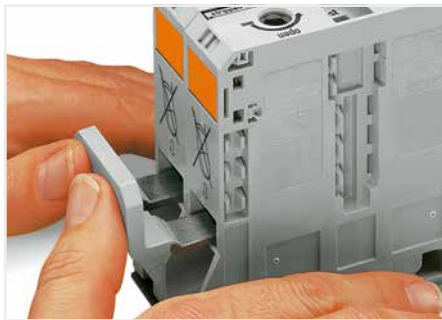
Commoning (50, 95 and 185 mm 2 ): Commoning with an adjacent jumper: insert the jumper above the conductor entry hole prior to conductor termination. The nominal cross-section remains unchanged.
