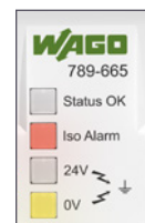
Ground fault 0 V
