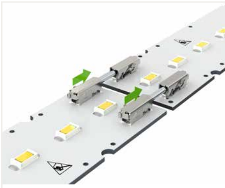
Assembly: Place PCBs on a flat surface and insert links into terminal blocks on adjoining PCBs. Disassembly: Open the terminal blocks with an operating tool (max. 5 mating cycles).
