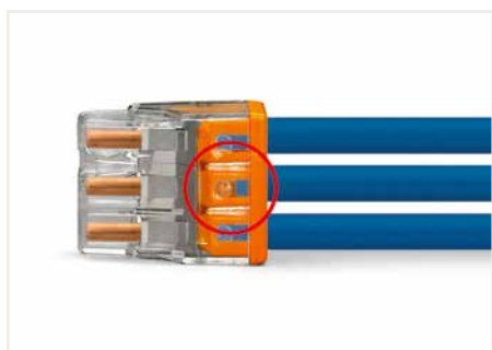
The transparent housing shows if conductors are fully inserted; within the colored base, a clear port shows if the conductor's strip length is correct. Conductors are correctly stripped if the clear port shows no bare conductor on the unprinted connector side. Picture shows center conductor with exceeded strip length.
