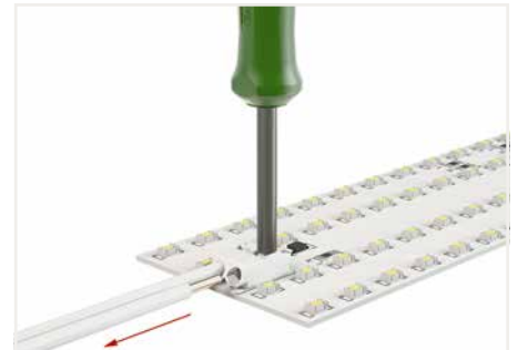
Insert/remove fine-stranded conductors by lightly pressing on push-button, e.g., via optional operating tool (206-860 or 2060-189).
