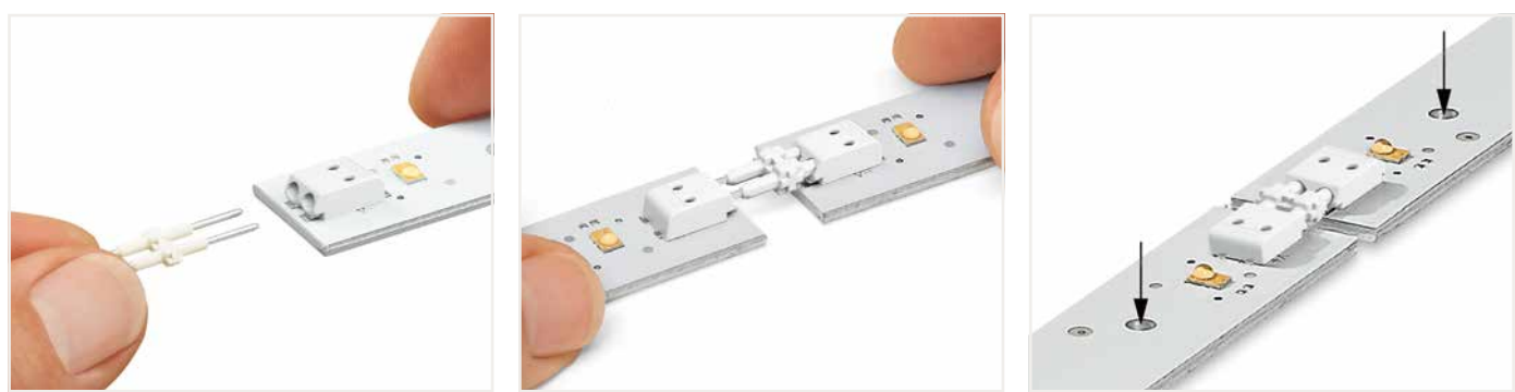
Inserting a board-to-board link into the terminal block. Assembly: Place PCBs on a flat surface and connect terminal blocks on adjoining PCBs via board-to-board link. Disassembly: Pull PCBs apart (max. 10 mating cycles). The PCBs must be secured.
