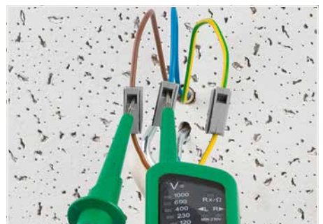
Testing via separate test ports.
