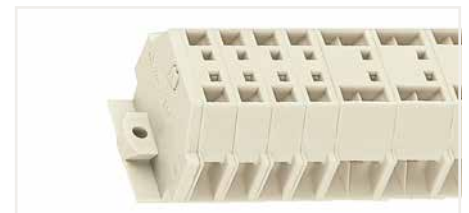
Terminal strip; with mounting flanges; for screw similar similar mounting types; 3.2 mm mounting hole diameter (with 209-123 Mounting Foot for DIN35 rail)
