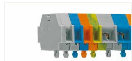
Terminal strip; with snap-in mounting feet; for 0.6 ... 1.2 mm plate thickness; 3.5 mm mounting hole diameter (also for 210-154 Aluminum DIN-Rail or with 209-120 Mounting Foot for DIN-35 rail)
