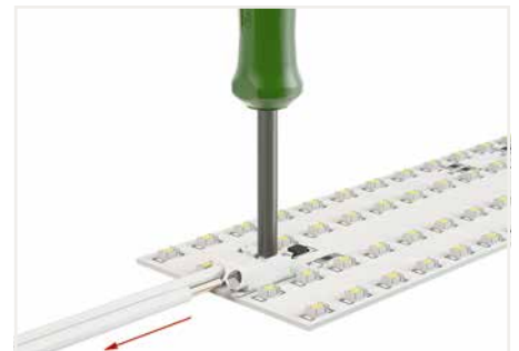
Insert/remove fine-stranded conductors by lightly pressing on push-button, e.g., via optional operating tool (206-866 or 2061-189).
