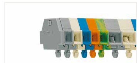
Terminal strip; with snap-in mounting feet; for 0.6 ... 1.2 mm plate thickness; 3.5 mm mounting hole diameter (also for 210-154 Aluminum DIN-Rail or with 209-120 Mounting Foot for DIN-35 rail)
