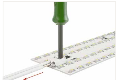
Insert/remove fine-stranded conductors by lightly pressing on a push-button, e.g., via operating tool (Item No. 206-861).
