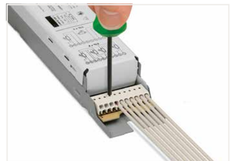
Removing a conductor via 1.0 mm Ø disconnection tool; (Item No. 206-841).
