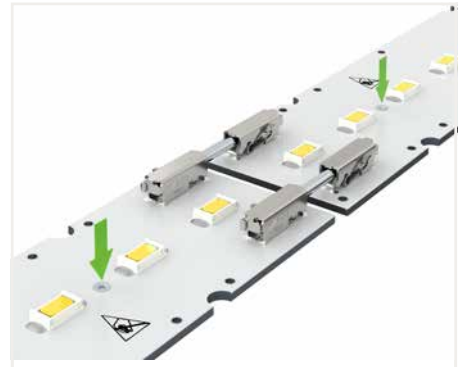
The PCBs must be secured.
