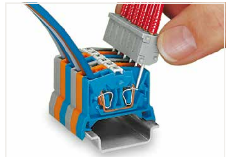
Testing by touch contact to the CAGE CLAMP® spring (limited to 0.5 A and 48 V test voltage) – test pins are not protected against accidental contact.
