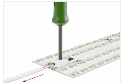
Easy conductor removal, e.g., via operating tool (Item No. 206-859, 2059-189) or "twist & pull" (max. 10 x, no reconnection of smaller conductors possible)
