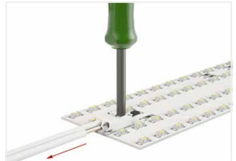
Insert/remove fine-stranded conductors by lightly pressing on a push-button, e.g., via operating tool (Item No. 206-860 or 2060-189).
