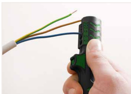
Stripping a wire insulation.
