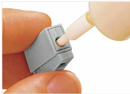
WAGO Lighting Connectors Push the "Alu-Plus" syringe's nozzle into the circular entry first and then into the square conductor entry hole of the WAGO Lighting Connector.
