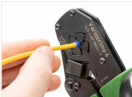
Squeeze handles until ratchet mechanism is released.
