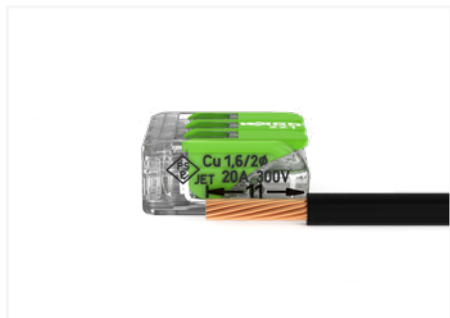
Strip conductor to 11 mm (0.43 inch).
