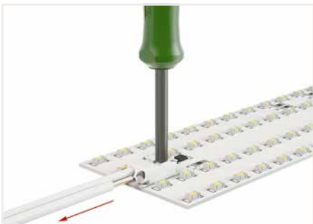
Insert/remove fine-stranded conductors – by lightly pressing on the push-button.
