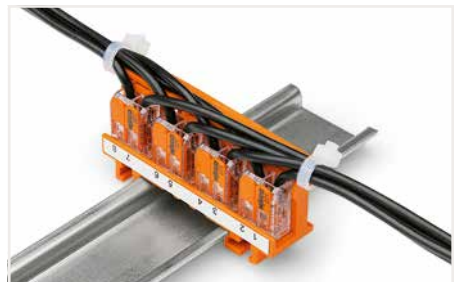
Strain relief via cable ties on the mounting carrier (transverse to the connectors' wiring direction); clamping units labeled via marking strips (210-334)
