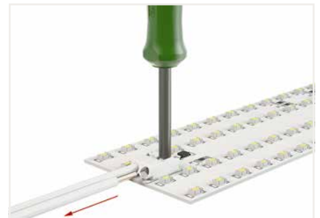
Insert/remove fine-stranded conductors by lightly pressing on a push-button, e.g., via operating tool (Item No. 206-860).
