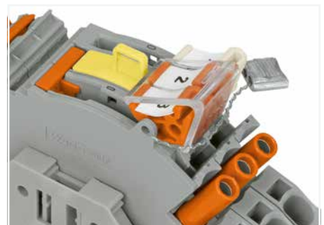
A lock-out seal can be used on the disconnect link in operating position I in combination with an end and separator plate (Item No. 2007-8893 or Item No. 2007-8894).
