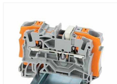
Step-down jumper (Item No. 2006-499) connects 6/4 mm 2 (10/12 AWG) terminal blocks (2206/2204 Series) with 4/2.5/1.5 mm 2 (AWG 12/14/16) terminal blocks (2204/2202/2201 Series).
