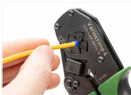
Squeeze handles until ratchet mechanism is released.
