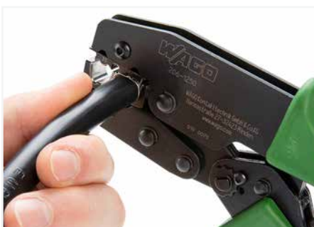
Squeeze handles until ratchet mechanism is released.
