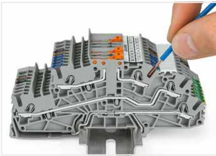
Inserting a conductor via push-in termination. Solid conductors with cross-sections from either one size above, or up to two sizes below, the rated cross-section can be simply pushed in – no tools needed.
