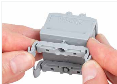
Terminal strip; with snap-in mounting feet Snapping a mounting foot (Item No. 209-120) (Distance between mounting feet: approx. 20 ... 25 mm)
