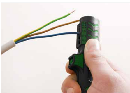
Stripping a conductor insulation.
