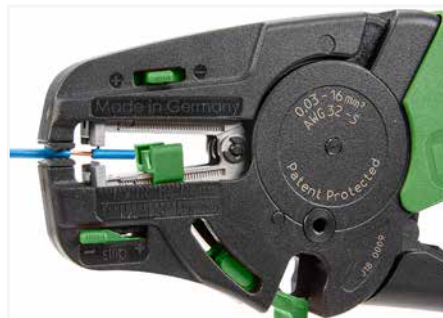
Partially stripping a conductor.
