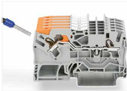
Push-in termination of fine-stranded conductors with ferrules
