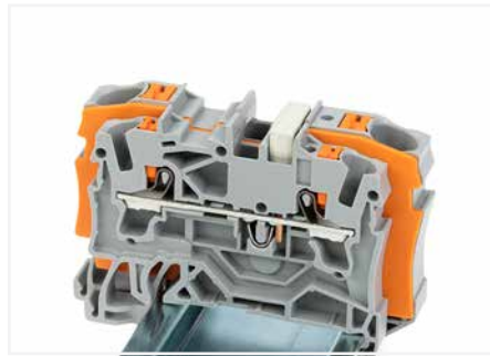
Step-down jumper (Item No. 2006-499) commons 6/4 mm 2 (10/12 AWG) terminal blocks (2206/2204 Series) with 4/2.5/1.5 mm 2 (AWG 12/14/16) terminal blocks (2204/2202/2201 Series).
