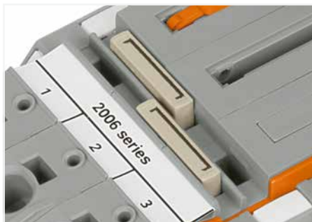
Commoning a 15 mm-wide terminal block via push-in type jumper bars: 1 to 3 (Item No. 2006-433) and 1 to 5 (Item No. 2006-435).
