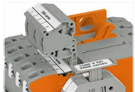
Alternatively, measurement can also be performed using Connectors (Item No. 2006-511) from terminal block 1 to 2. Spacer modules (Item No. 2006-549) must be used to compensate for the 15 mm terminal block width.
